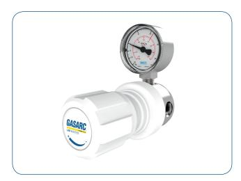
The Lab Master LGL500 Series single stage diaphragm line regulators are designed for secondary pressure gas control of non-corrosive or toxic, high purity gases up to grade 5.0 purity (99.999%), on gas distribution systems.
