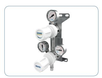
The Lab Master LGX5000 Series two stage diaphragm switch change gas control panels are designed for the primary control of non-corrosive or toxic, high purity gases up to grade 5.0 (99.999%), on gas distribution systems where a constant delivery pressure is required.
