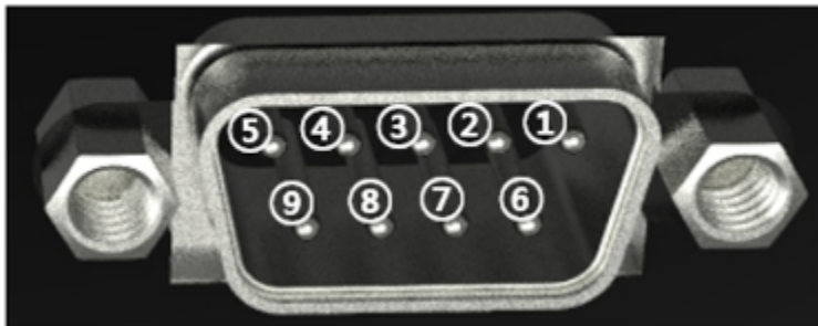
Model WIZ-801 Connector - 9 Pin male D-Sub Connector
